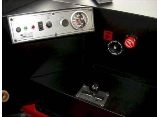
7. Wire up the fan and water pump. The water pump should be wired so that anytime the ignition is on, the pump is on. This is the best way to ensure that the pump is always running whenever the engine is on. The fan should be on a circuit with a 30 amp fuse. A 20 amp fuse may not be enough – especially if you have other fans on the same circuit.
