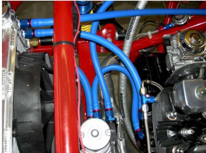
6. Install the adapter and temperature gauge probe in the radiator. Run the lines back to the interior of the car and install the water temperature gauge. One good location is where the tach recall used to go, as shown to the right. The tach recall can be placed on the side panel below the fan switches.
