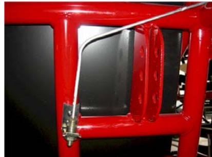
3. Attach the “T” shaped brake line to the quick change rearend by drilling a small hole as shown in the photo and attach with the enclosed allen bolt and nylock nut.
