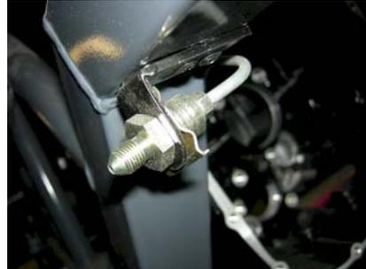
Rear brake line run from the union up front, around to the mounting tab in the rear of the car
