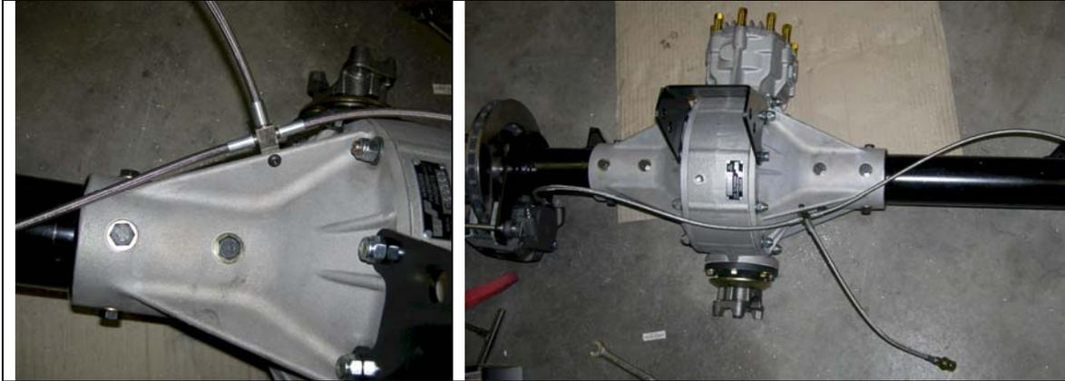
4. Now the hard work is done. To complete the job, simply attach the enclosed hardline to stainless adapters to the mounting tabs using the enclosed brake clips. If the fit isn't secure, you may need to slightly bend the tabs of the brake clip using pliers.
